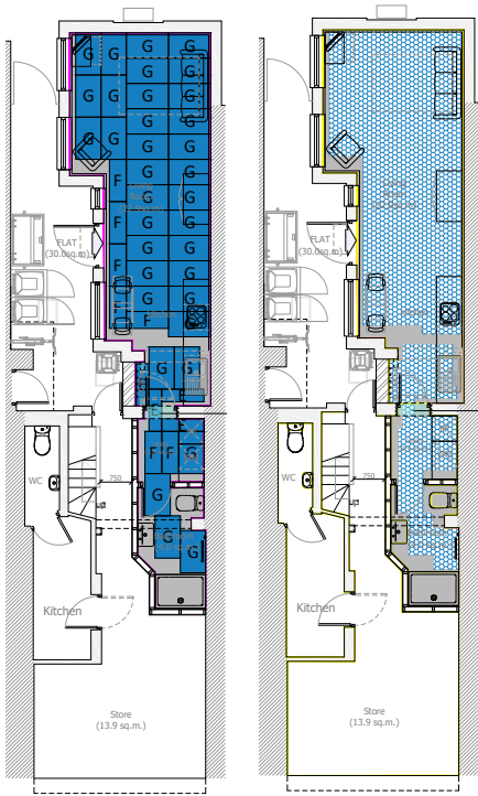
A typical design layout, showing the Quantum boards fitting in to the floor shape.
